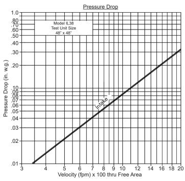
Intake air converted to standard air density.
